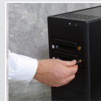
Insert carrier into frame, turn key lock & press power button
