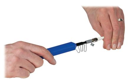
Open the cover on the guide cap, and insert the fibre connector over the guide cap. Push the case to start the cleaning process; a click indicates that the cleaning is complete.
