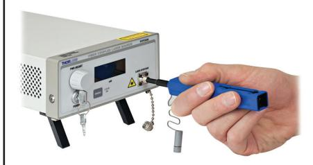
Remove the guide cap completely from the device, and insert the tip of the cleaner into the bulhead connector. Push the case to start the cleaning process; a click indicates that the cleaning is complete.
