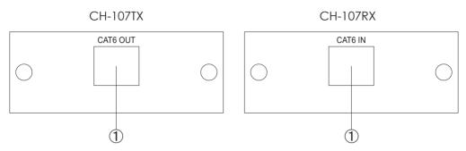
① CAT6 OUT/IN: Connect the CAT6 output of the transmitter with a CAT6 cable to the CAT6 input of the receiver.
